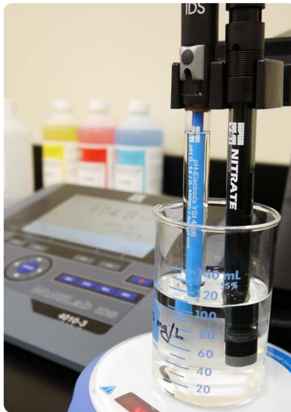
Ideal set-up for calibration. A stir plate, 150 mL glass beaker, temperature sensor (e.g. from pH electrode), ISE instrument, and ISA are all used.
