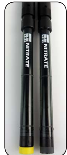
Nitrate electrode with blank sensor module (left) and electrode with sensor module (right) installed.
