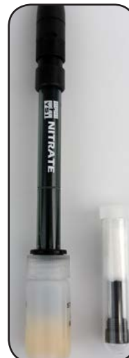
Nitrate electrode with blank sensor module installed and sensor module in dry, glass vial.
