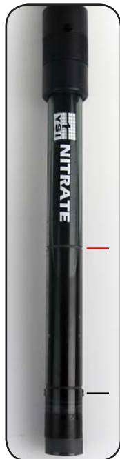
Location of inner junction (red line) and outer (black line) reference junctions.
